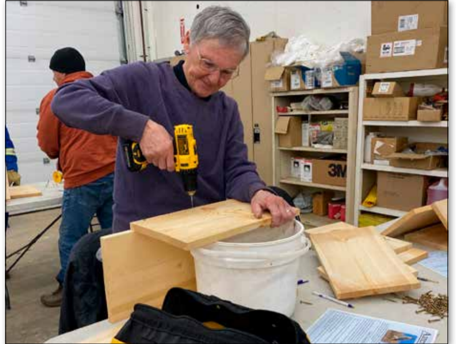
Vi uses a pail as a second set of hands for straight construction.
