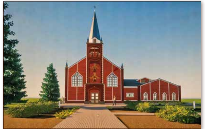
Designs for the new St. Jean Baptiste Church show a modern church with a traditional design. The bell tower will stand 75 feet above 100 Avenue and is separated from the church proper to allow the bells to ring clearly once again.
