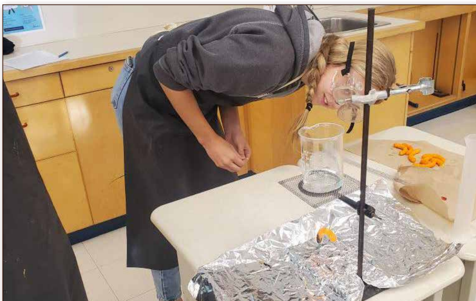
In order to determine the number of calories in a cheese puff, H.A. Kotash School students in Smoky Lake conducted a calorimetry experiment in their Chemistry 30 class. Students placed a known mass of cheese puffs into a container of water and measured the temperature change that occurred. From this, students were able to calculate the number of calories in each cheese puff.
