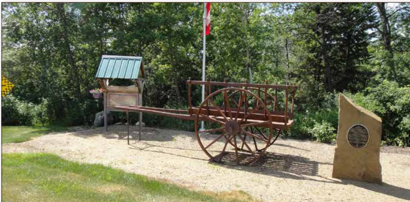
"This cart with high wheels was an excellent and convertible way of transportation. It could be pulled by horses or oxen and could load 1000 lbs. Due to the high wheels, it would make it through deep mud. In the case of river crossings, the wheels would be removed, and it would float like a raft".
